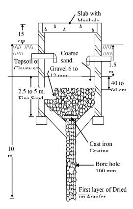
Figure 3. Recharge Bore-Well
